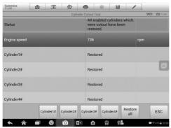
Figure 5-17 Sample Cylinder Service Screen 4
