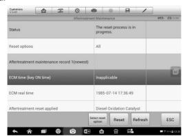
Figure 5-3 Sample Oil Reset Service Screen 1
