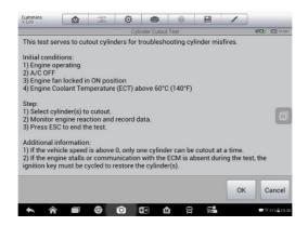
Figure 5-14 Sample Cylinder Service Screen 1
