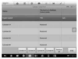
Figure 5-15 Sample Cylinder Service Screen 2
