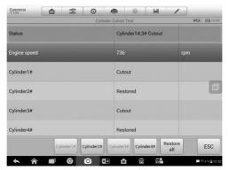
Figure 5-16 Sample Cylinder Service Screen 3
