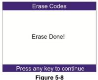
• If the codes are not cleared, then an "Erase Failure. Turn Key on with Engine off!" message appears.
